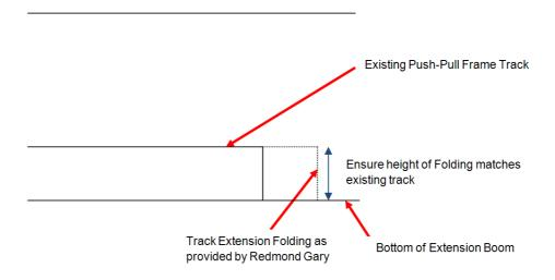
Step 3: Once the height has been set and the folding is ready to be positioned into place, remove the galvanising from the top surface of the track in the middle about 40 mm in length for the weld to adhere to whilst also grinding the mating surface on the track extension folding.
