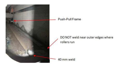
**Step 6:** If deemed necessary, a tack weld can also be placed on each front corner to prevent the folding from lifting, although this is unlikely.
