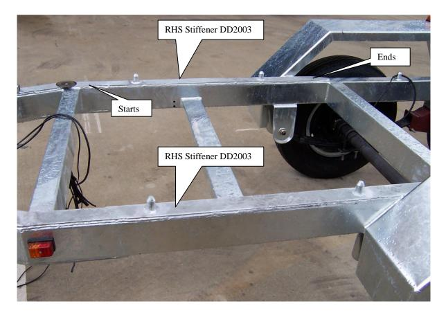
Note: Some trailers have fixed drum frames and others have removable drum frames as illustrated here. In both cases this stiffener is required.
