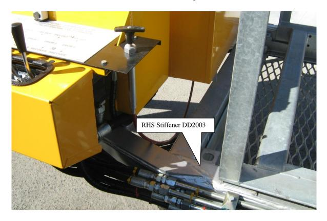
Machine owners must immediately implement an inspection of the Front Suspension hanger welding and the electrical access hole directly under the front of the mudguards. If there is any sign of cracking, the trailer is to be withdrawn from service until repair and the additional RHS stiffeners added.
