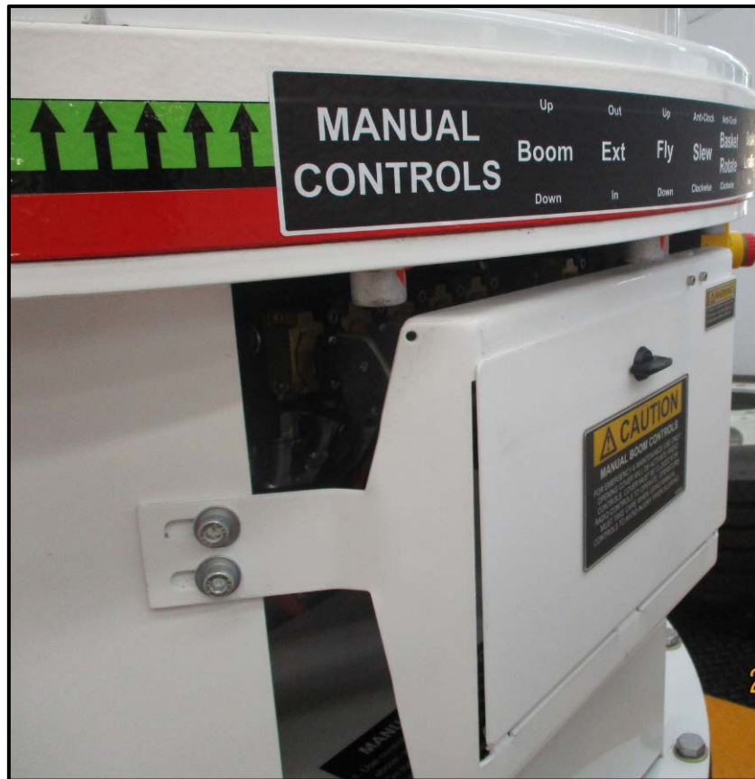
Figure 1: Turret Manual Controls station on MEWP deck
