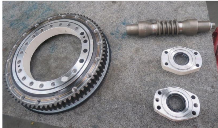
Figure 2 - Disassembled RG worm gear drive
