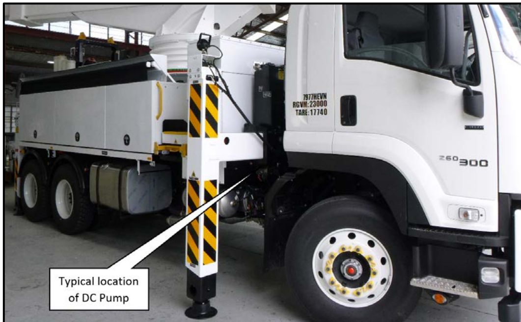
Figure 1: Typical DC Pump location on MEWP
