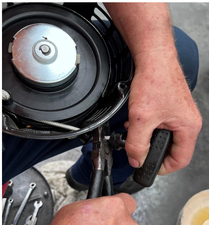
Figure 9: Removing the pull start handle
