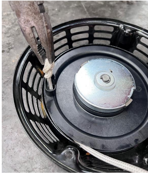
Figure 10: Pull cord removal
