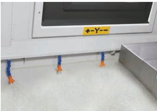
Chassis Chip Flushing
