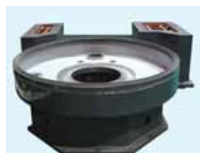
One-piece machine base with built-in gearbox and spindle
